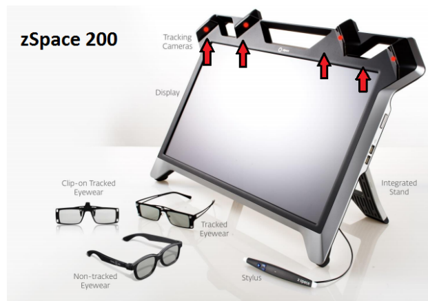
Figure 5. Major components of the zSpace platform
